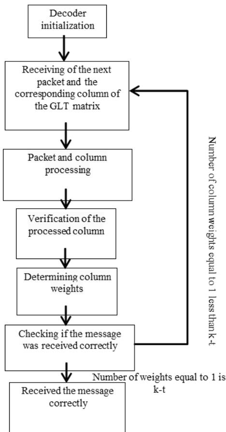
Figure 2: Procedure of pipeline processing.
