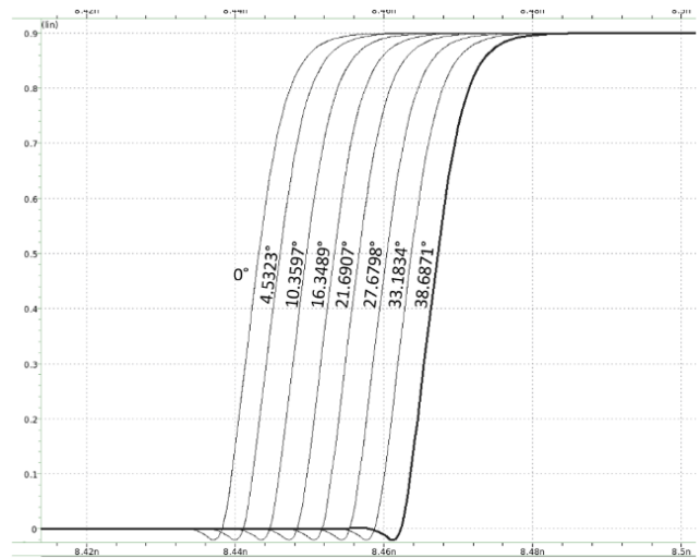
Fig. 12 8-step interpolation between two phases.
